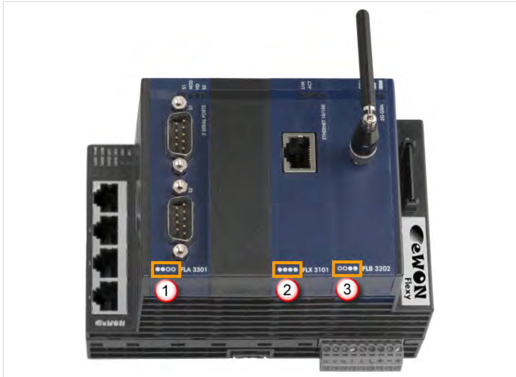
Fig. 16 Slot Compatibility Markings
